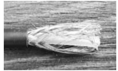
3/4 inch of outer insulation removed from the end of a length of RG-58 coax cable
