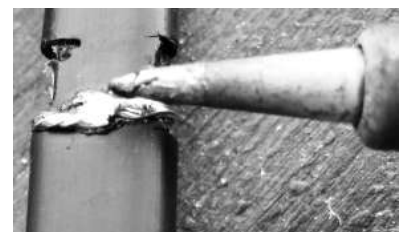
Wires overlapped and soldered
