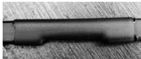
The gap with heat shrink in place.
