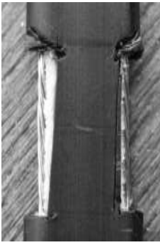
Tap point with insulation removed
